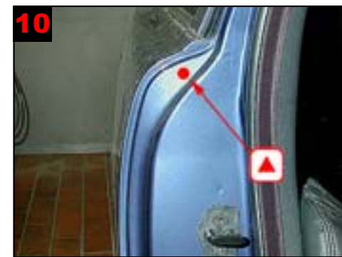
10 C-pillar/rear wing: Fig: drilling at correct level.
