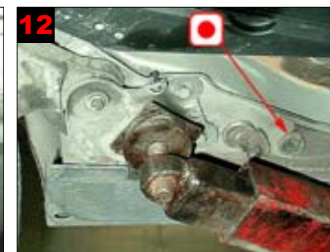
12 Longitudinal member after wheel arch rear: Treat via 1 drilled hole and existing plugged hole.
