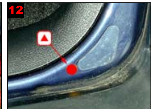
12 Rear panel: Fig: drilling at correct level.
