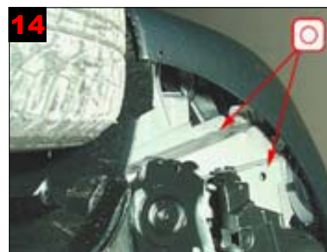
14 Longitudinal member front: Treat via existing holes.
