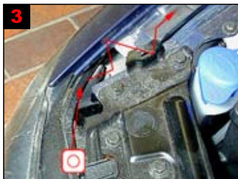
3 Front wing: Treatment of top member in wing via existing gap.
