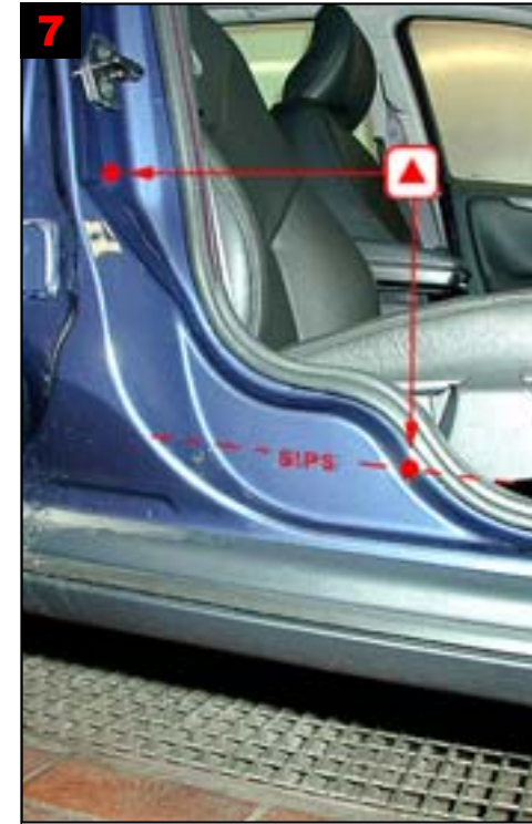
7 B-pillar: Treat via 2 drilled holes. Lower drill hole level with SIPS-logo.
