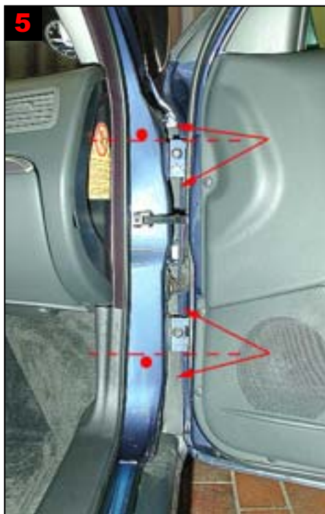
5 A-pillar and front wing: Treat via 2 drilled holes. Drill level right above and right below door hinges. Treatment of front wing with lance, from clearing between A-pillar and wing/door.
