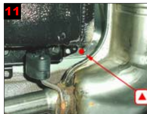
11 Longitudinal member rear: 1 drill hole each side through cover plate.
